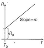
The temperature coefficient  $(\alpha)$  of the conductor is
